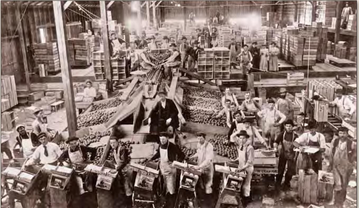
Ontario Fruit Association had electric lighting from Sierra Power Plant, though they did not have three-phase power as their sizing machine was powered by men. Observe the two men facing each other seated on top of the sizing machine. They operated the treadmill. The growing California citrus industry was ready for modernization! (circa 1902).
